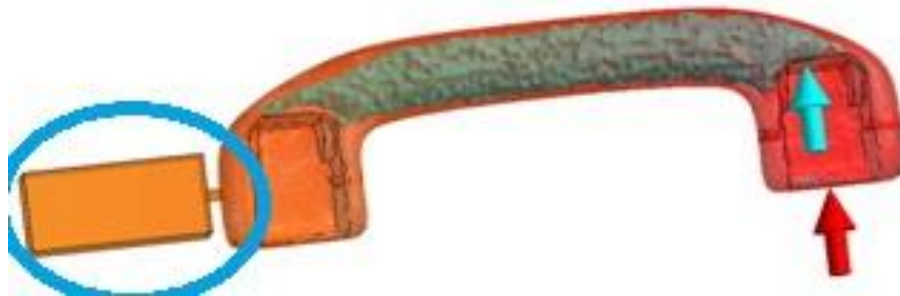
GAS INJECTION OVER FLOW
